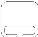
Detachable plates assembled onto belt's width to locate product.
