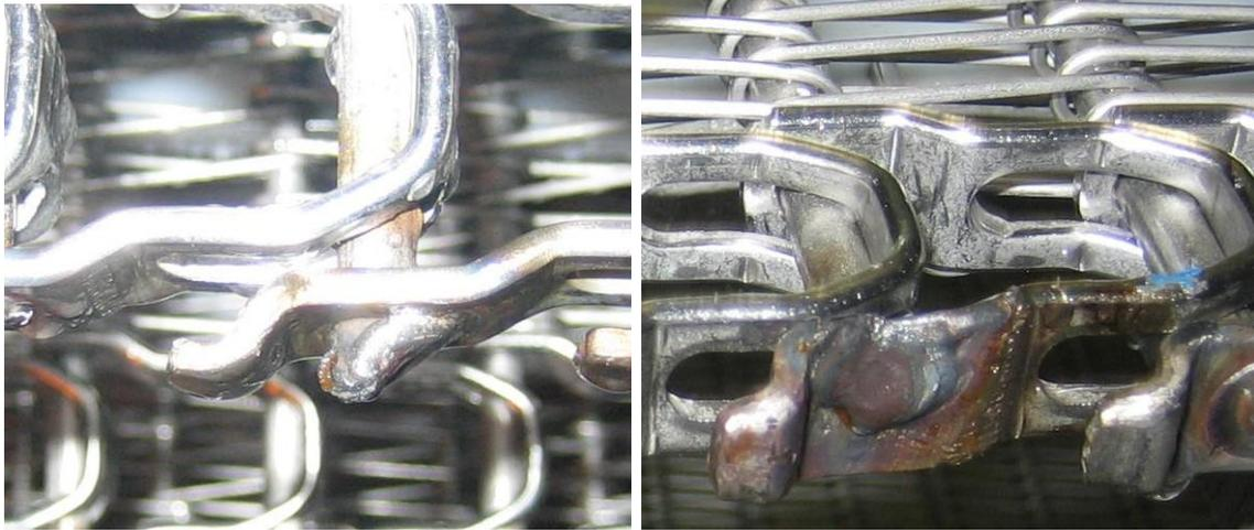
*Two more examples of bad welds. On the left, the rod has not been melted into the link and sticks beyond the link's protrusion leg. On the right the weld is below the surface of the link and has burned the link material away.*
