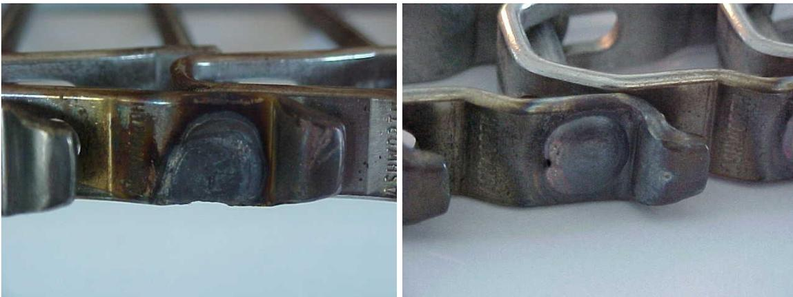
*Above are examples of poor welds. The weld on the left has burnt through the link while the weld on the right has not completely filled the hole in the link.*
